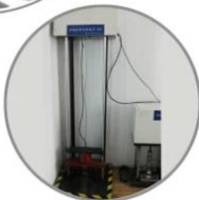
Impact Resistant Testing Machine
