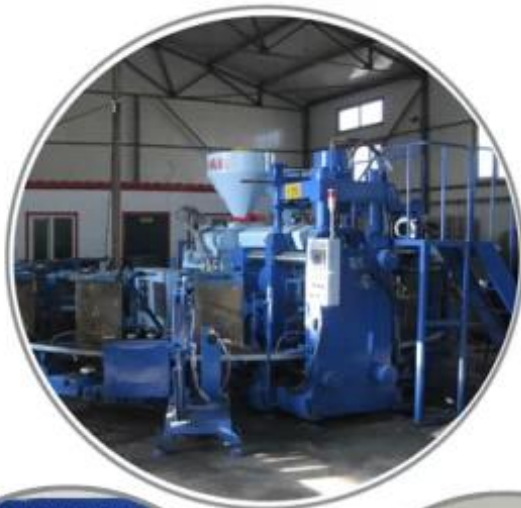
Automatic Injection Molding Machine
