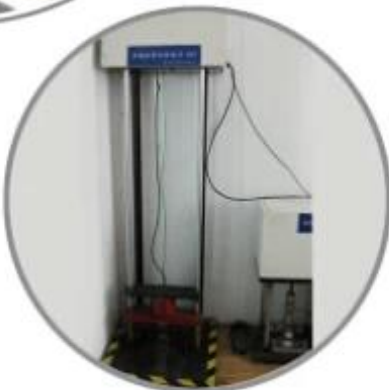
Impact Resistant Testing Machine
