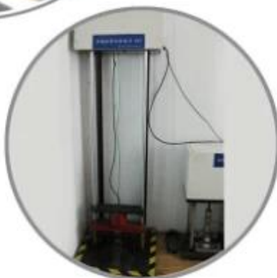
Impact Resistant Testing Machine
