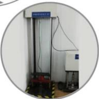
Impact Resistant Testing Machine
