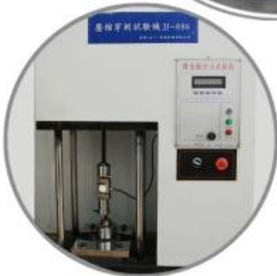
Puncture Testing Machine
