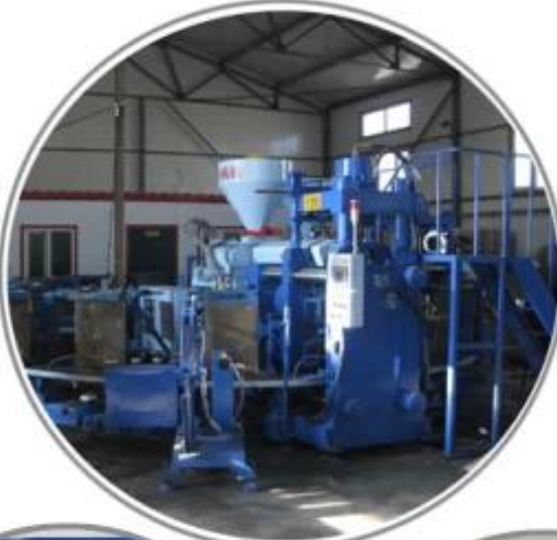
Automatic Injection Molding Machine
