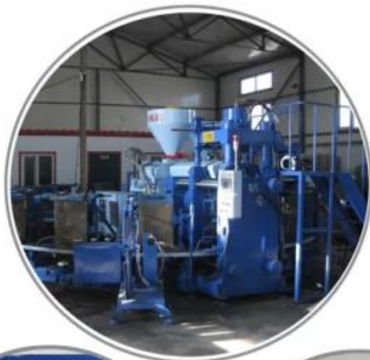
Automatic Injection Molding Machine
